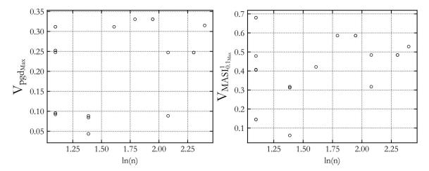
Figure 11: Distribution of the variability inside a radius of 3 km for left) PGD and right) Modified Acceleration Spectrum Intensity MASI – 1
