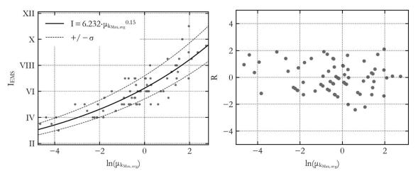
Figure 28: Test on max distance = 0.5 km – equation b: Kinematic ductility  $\mu_{max}$ : regression line (left) and variation of residuals (right)
