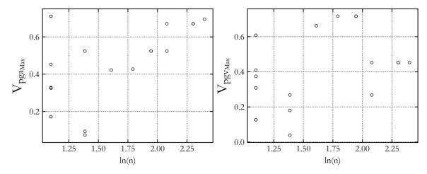
Figure 10: Distribution of the variability inside a radius of 3 km for left) PGA and right) PGV
