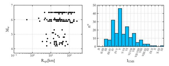
Figure 23: Magnitude vs Epicentral distance of the records included in the final dataset (left) and Distribution of couples MDP-record for each intensity degree (right)
