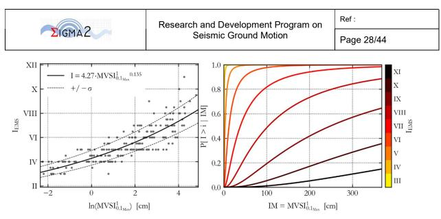
Figure 19: Modified Velocity Spectrum Intensity *MVSI – 1*: variation of residuals (up-left), their distribution (up- right), regression line (down-right) and "fragility" functions (down-left)
