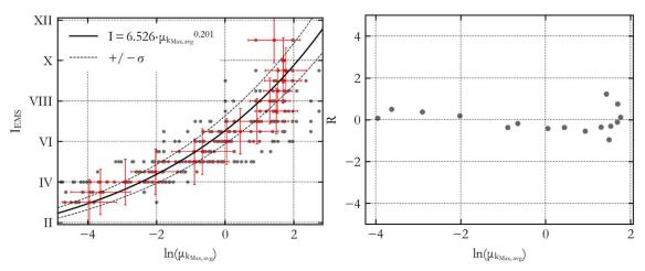
Figure 26: Test on binned data – equation b: Kinematic ductility  $\mu_{max}$ : regression line (left) and variation of residuals (right)
