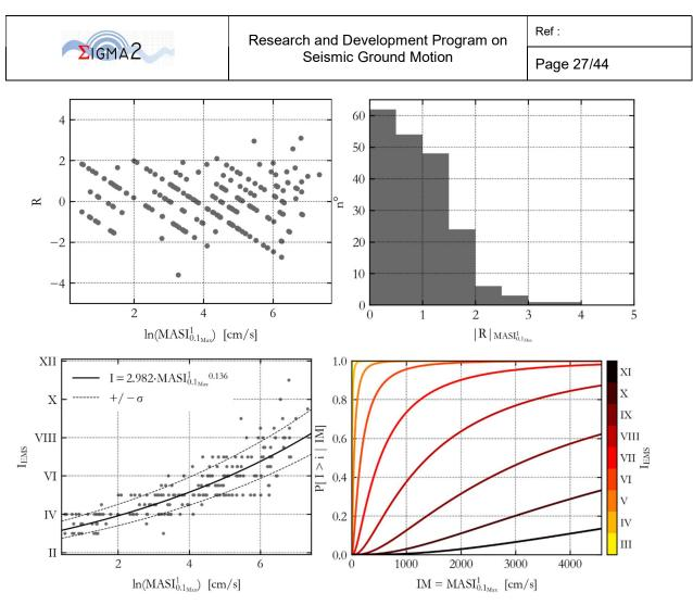
Figure 18: Modified Acceleration Spectrum Intensity *MASI* – 1: variation of residuals (up-left), their distribution (up- right), regression line (down-right) and "fragility" functions (down-left)
