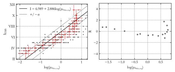
Figure 25: Test on binned data – equation a: Kinematic ductility  $\mu_{max}$ : regression line (left) and variation of residuals (right)
