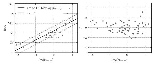
Figure 27: Test on max distance = 0.5 km – equation a: Kinematic ductility  $\mu_{max}$ : regression line (left) and variation of residuals (right)
