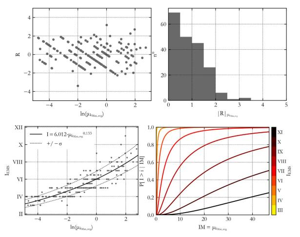
Figure 20: Kinematic ductility  $\mu_{max}$ : variation of residuals (up-left), their distribution (up- right), regression line (down-right) and "fragility" functions (down-left)
