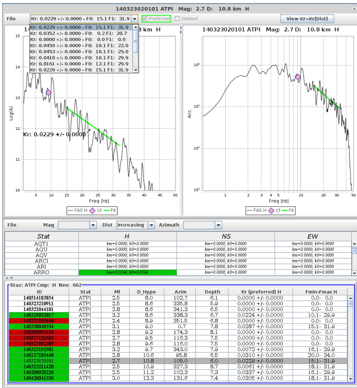
Figure 1. Example of application of the tool adopted to estimate the k parameter: the horizontal Fourier spectra of a M 2.7 earthquake at IV.ATPI station is plotted in lin-log (left) and log-log (right) scale. The diamond pink is the theoretical corner frequency; the green line is the fitted model visually selected; the k values estimated in the other frequency band is also reported.
