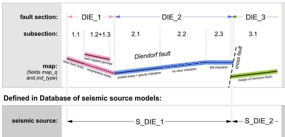
Fig. 3.2.1: Schematic illustration to explain the concept used for description of a fault in the Analytical fault map of Fault database (top). Note that the seismic sources (including proved or hypothetical earthquake segments at capable faults) are defined in Model of seismic fault sources (MSFS; bottom).
