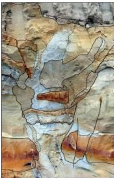
Detail of sand blow (structure A in the profile). From Špaček et al. (2018), modified.
