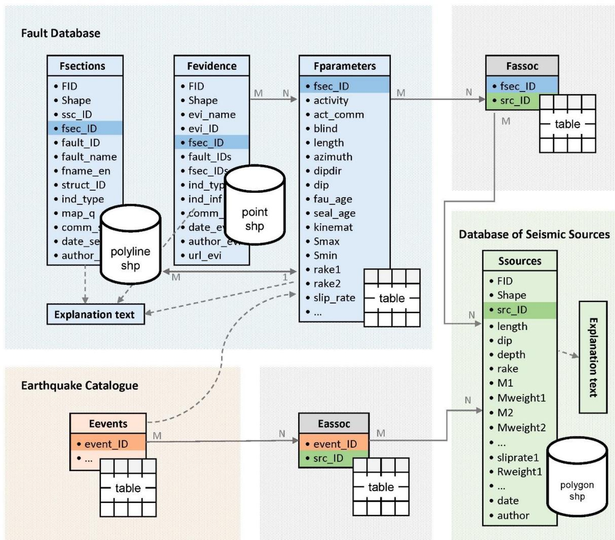
Fig 2.2. Schematic representation of basic intended structure and linking of the databases for Earthquake catalog, Fault database and Database of seismic sources. Connecting fields are highlighted. Shp – ESRI shapefile.
