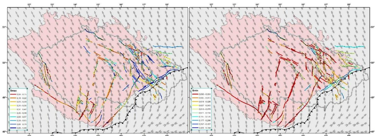
Fig. 3.4.1. Fault maps with color-coded maximum (left) and minimum (right) values of fault stability coefficient  $S$ . Variance of maximum stress orientation in the stress models used is shown schematically by grey arrows.
