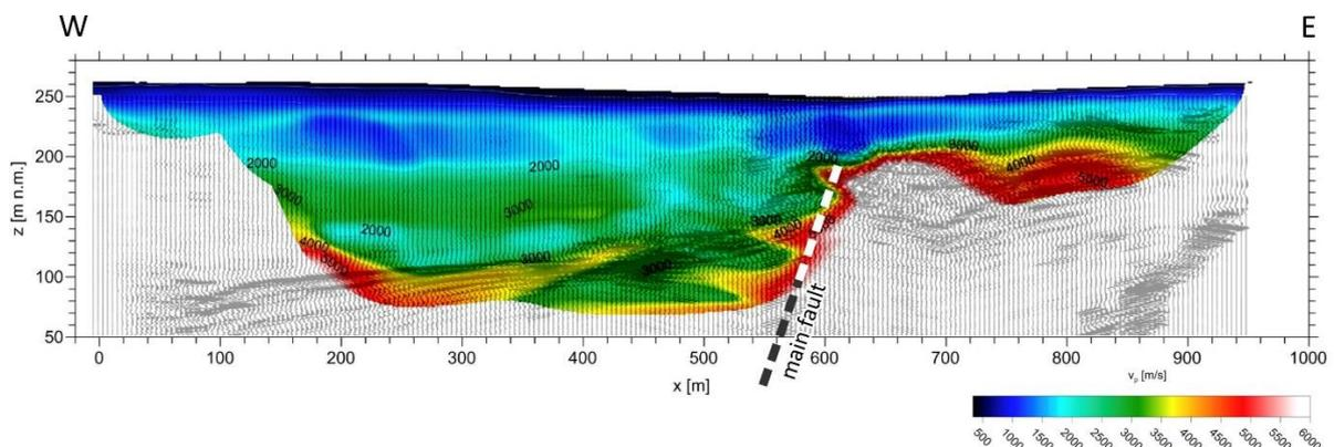
Stack of SRT and seismic reflection profiles near Lesonice. Modified from Alexa 2017.
