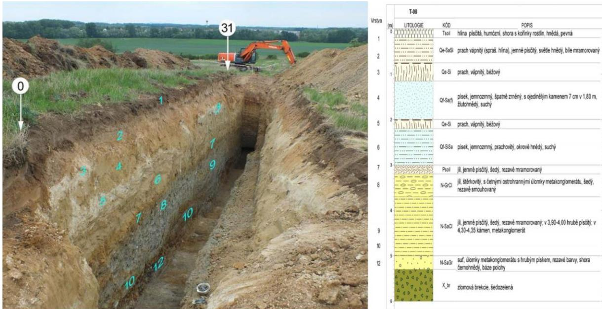
Trench RTAS-3 and stratigraphic scheme of exposed sequence of sediments covering the faulted bedrock. From Prachař et al. 2017, modified.
