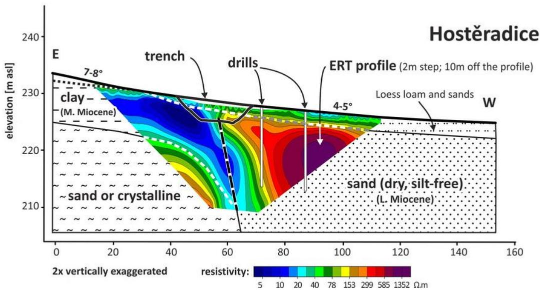
Hostěradice profile with ERT, interpreted geology and position of the trench. Note vertical exaggeration. From Špaček et al. 2017.
