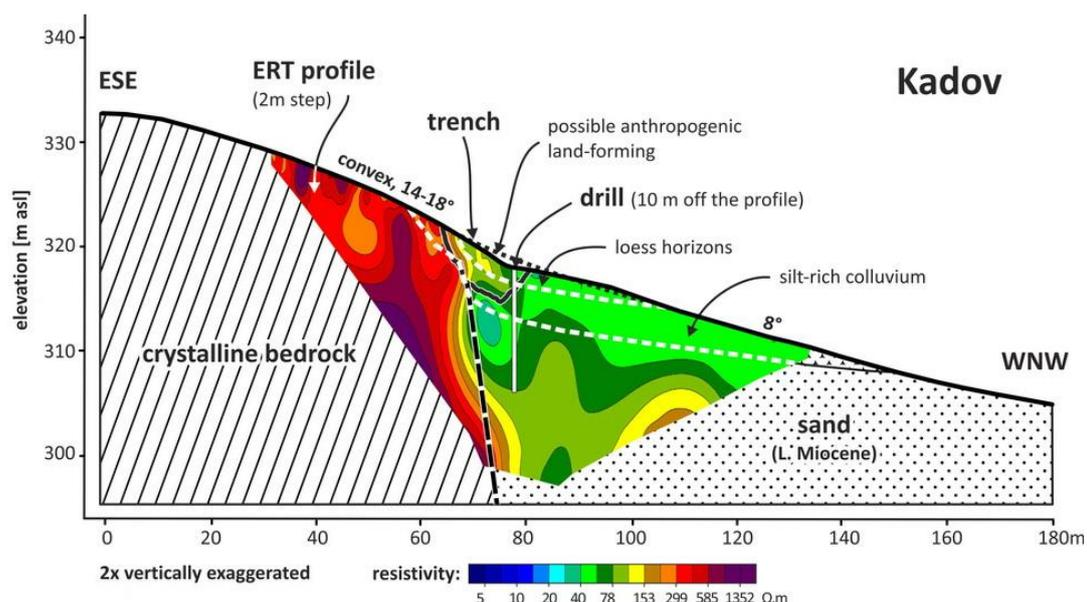
Profile Kadov with ERT, interpreted geology and position of the trench. Note the vertical exaggeration. From Špaček et al. 2017.
