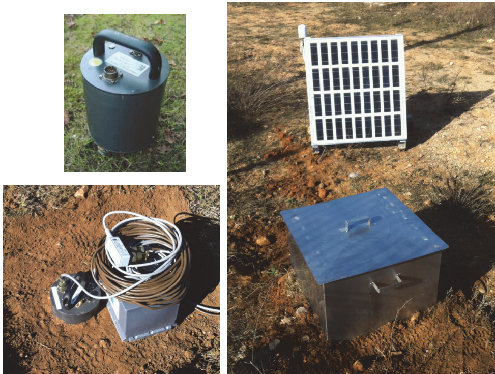
Figure 1: Typical installation of a CMG6-TD broadband sensor on "site A". Top-left: the seismometers before installation; bottom-left: the seismometer buried and connected to power supply; right: the battery and seismometer are protected by a stainless steel coverage with thermal insulation, the system is powered by a solar panel.
