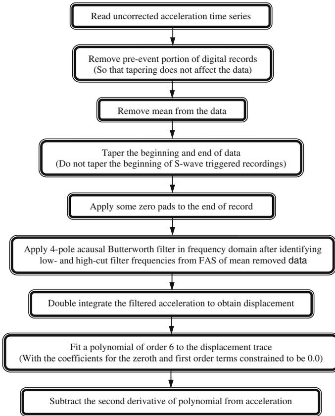
**Fig. 4** Band-pass filtering and post-processing scheme (after the removal of existing non-standard errors) used in RESORCE (modified from Boore et al. 2012). The original version of the implemented procedure is given in Chiou et al. (2008)
