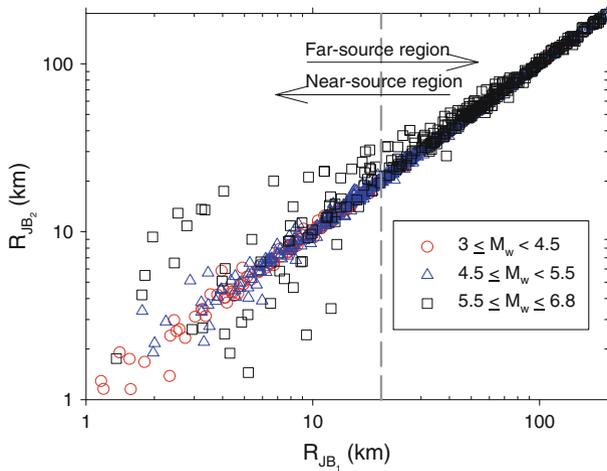
**Fig. 2** Differences between  $R_{JB_1} - R_{JB_2}$  pairs computed from the two planes given by the double-couple fault-plane solutions in the absence of extended-source distance measures ( $R_{JB}$  and  $R_{rup}$ ) in the reference source databases. *Different color codes and symbols indicate different magnitude intervals*
