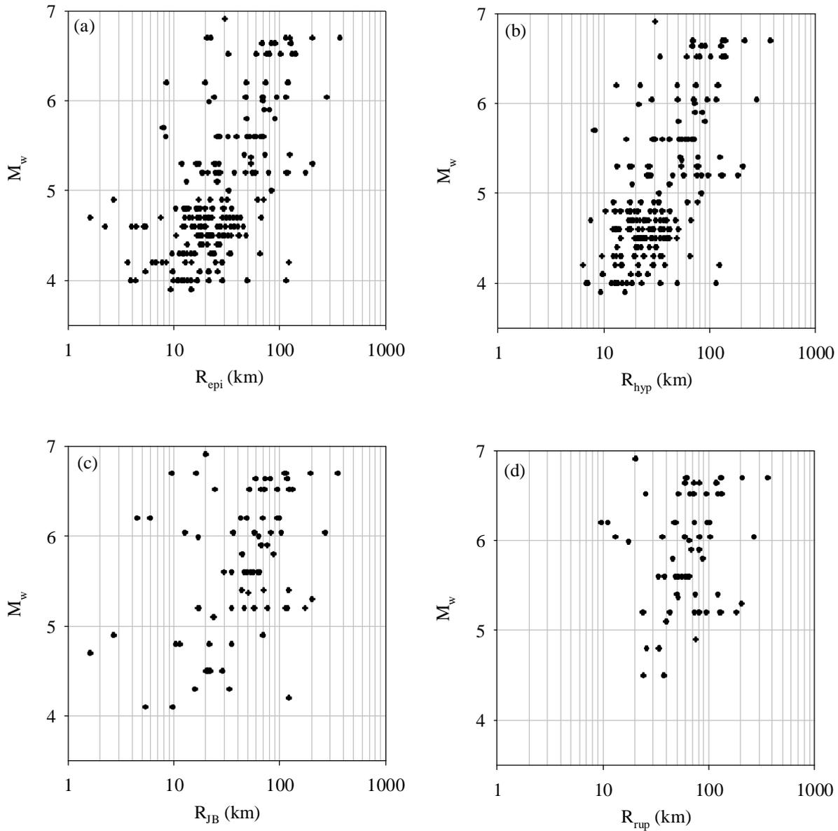
Figure 1. Scatter plots of Greek data for  $M_w$  vs. (a)  $R_{epi}$ , (b)  $R_{hyp}$ , (c)  $R_{JB}$  and (d)  $R_{rup}$ .
