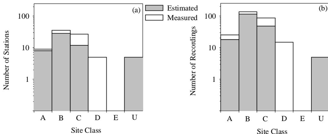
Figure 4. Greek (a) station and (b) recording distribution as a function of site class. The nomenclature used for site classes is adopted from Eurocode 8 (CEN, 2004). A site class is  $VS_{30} \geq 800$  m/s, B site class is 800 m/s
