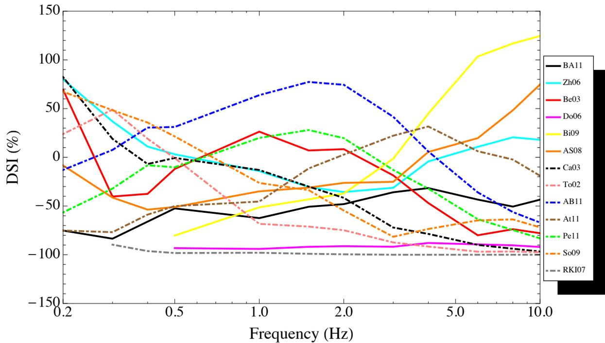
Figure 7: DSI values against response spectra frequency for the GMPEs that get higher LLH values.
