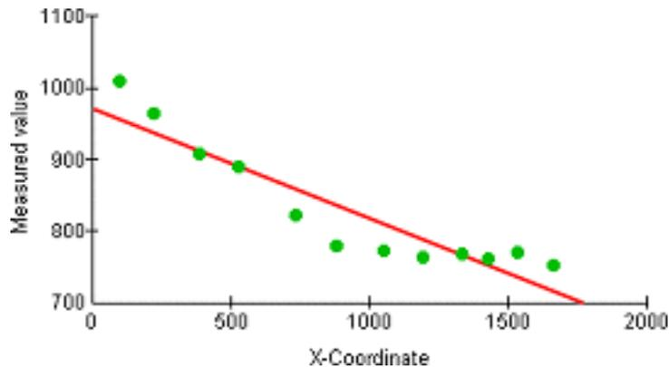
Figure 3: A first order global polynomial surface in cross-section. The surface (red line) captures coarse-scale pattern in the data. It does not pass through the sampled data (green points).
