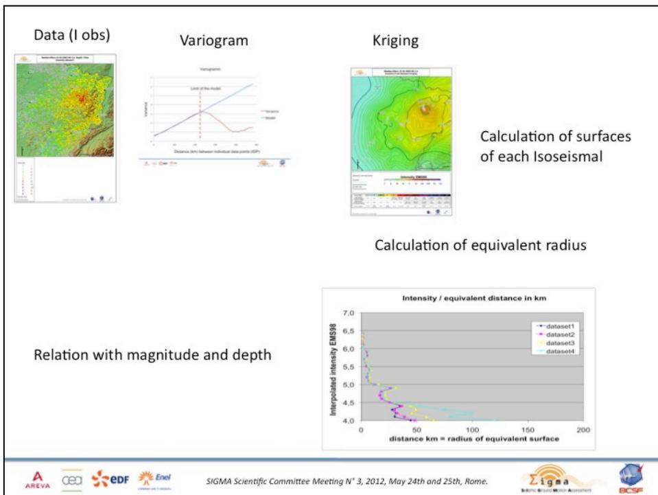
Figure 27: Schema of the kriging method until area estimation
