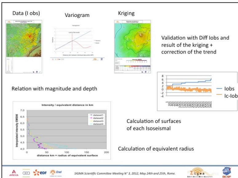
Figure 29: Schema of the kriging method, until area estimation, including the tendency correction
